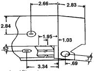
All knockouts are 7/8 inch diameter for 1/2 inch conduit.
